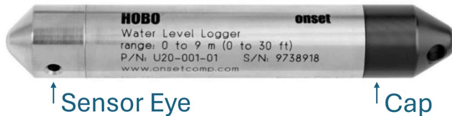
Figure 19 An Onset HOB0 U20 Water Level Logger. This is a standard model meant for water up to 9 metres above the sensor eye. The sensor eye where the water pressure is measured and the cap covering the communication port are marked for reference. The titanium models are nearly identical in appearance, aside from the markings identifying them as being titanium.
