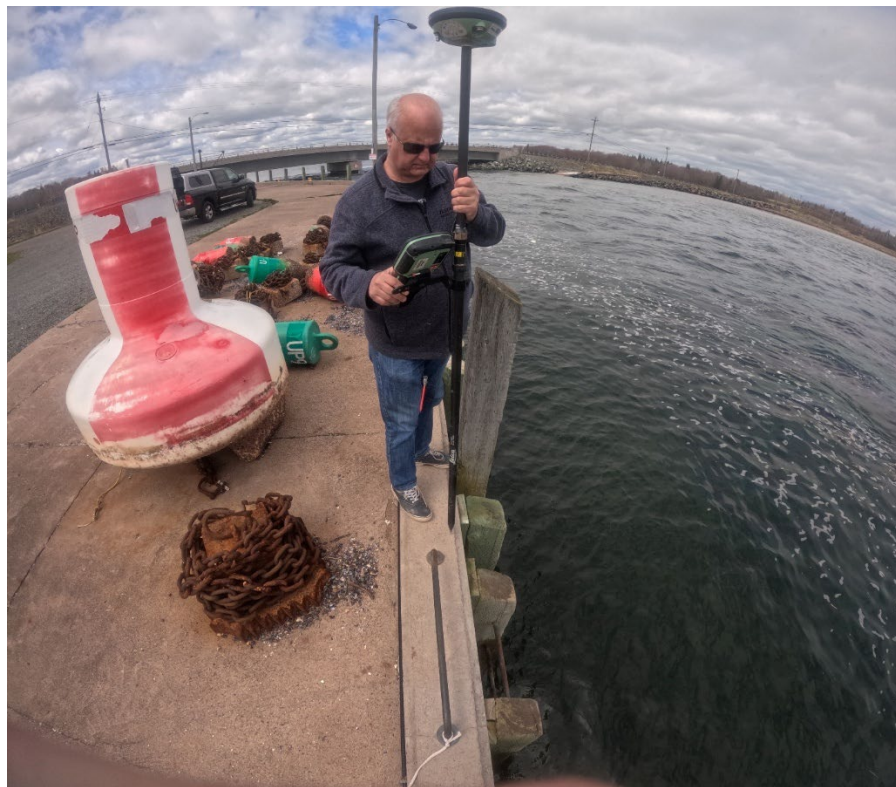
Figure 22 Colleague Sean Dzafovic collecting the GNSS reference point for the Northport Wharf.
