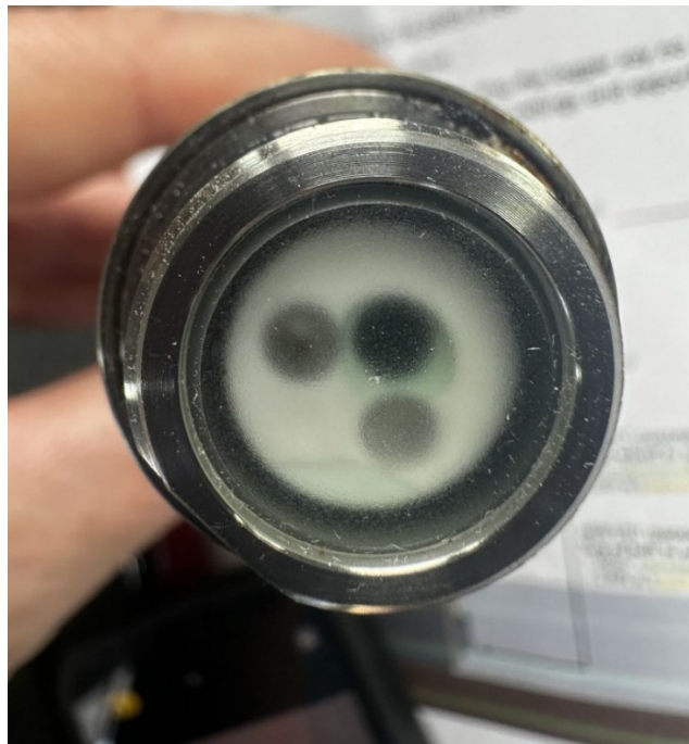
Figure 27 Damaged MCC logger, as seen in email correspondence with Maggie Pitts in July 2025.
