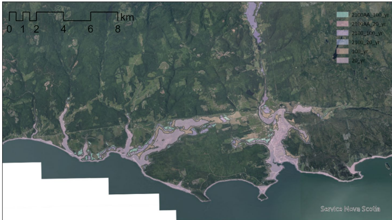
Figure 37 Example of coastal flood hazard layers near Parrsboro on the Bay of Fundy for 1-20 and 1-100-year events today and in 2050 and 2100.
